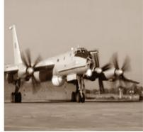
seidon aircraft. The TU-142MKEis a 53.08-meter-long aircraft with a 50-meter wingspan and a height of 12.12 meters. Weighing 90,000 kg, it could take off with a maximum weight of 185,000 kg, according to the statement. Similarly, the Westland Sea King MK42B helicopter played a key
