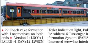
LSLRD+4 LWS+12 LWSCN +4 LWS +1 LSLRD+LOCO • Version version 2: LOCO+1 LSLRD+5 LWS+4 LWSCN+1 LWCD+4 LWSCN+6 LWS + 1 LSLRD + LOCO • Speed Potential: 130 kmph • Control couplers on end walls for push-pull operation with locos at both ends for high acceleration Semi permanent couplers for jerk free travel
